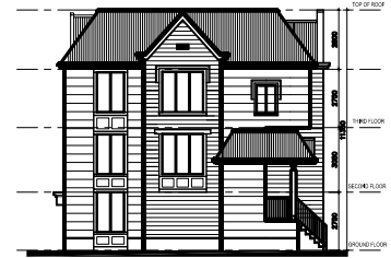
Buildings "3"- West Elevation
