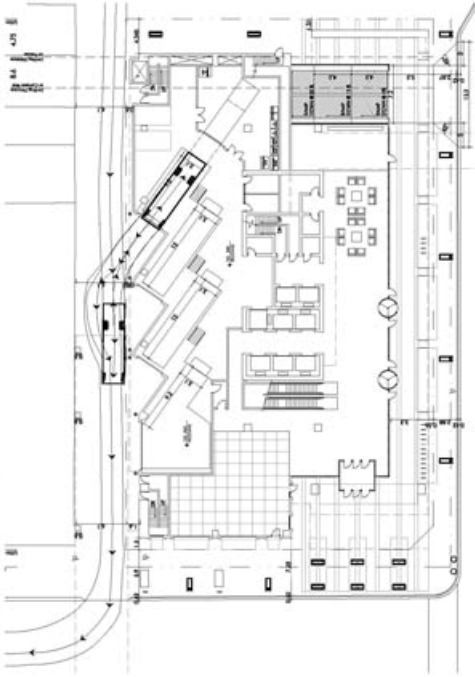
1. TYPICAL 8m CORNER TYPE TRUCK LOADING DIAGRAM
